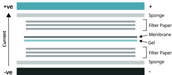
Figure 7. A schematic representation of protein transfer from the gel to a membrane. Negatively charged proteins move up towards the positive cathode and onto the membrane.
